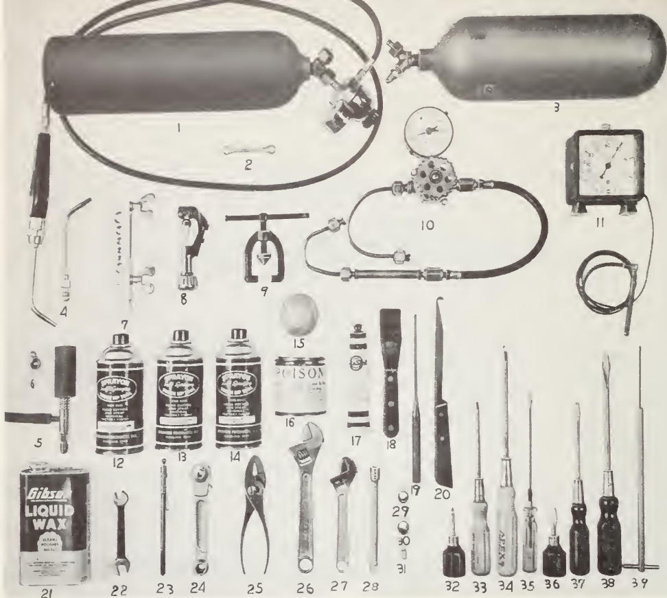
11-2. A typical set of tools needed for servicing operations. (Gibson Refrigerator Co.)
